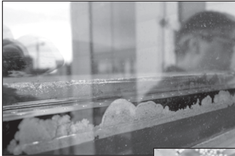
Figure 25 – Corrosion of partially edge-deleted low-e coating.
