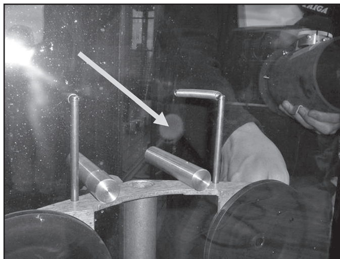
Figure 15 – Complaints of dirt build-up and fingerings on the inside of IGUs prompted dew point testing, which revealed high levels of moisture inside the units.
