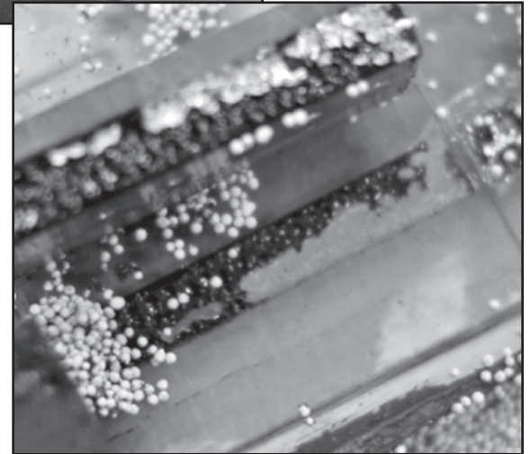
Figure 26 – Low-e corrosion residue left on IGU sealant after pull test showing loss of adhesion.
