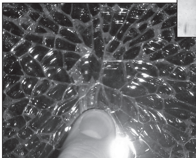
Figure 11 – Typical butterfly pattern at the epicenter of the break with magnified NiS inclusion inset (right).
