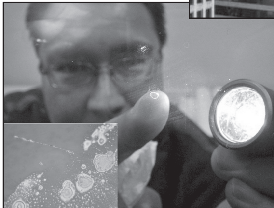
Figure 18 – One of the authors examining damage to low-e coatings caused by volatile fogging and condensation fogging. Same location under magnification shows corrosion pattern (inset).
